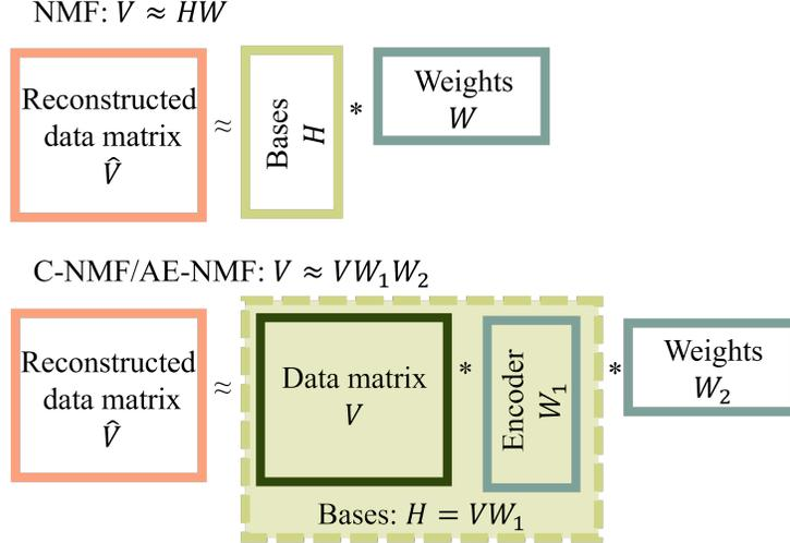
Figure 1: Schematic representation of the composition of basis vectors and weights in NMF (top) and C-NMF and AE-NMF (bottom).
