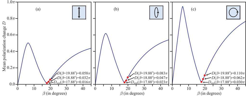
Fig. 9. Dependence of  $D$  on the base angle  $\beta$  at  $n_M = 0.1568 + 3.8060i$  for three different states of polarization. (a) incident field with vertical polarization, (b) incident field with elliptical polarization, and (c) incident field with circular polarization.
