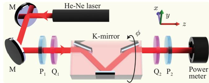
Fig. 5. Schematic of the experimental setup for measuring transmitted states of polarization using the home-built K-mirror at various rotation angles  $\phi$ . M : Mirror;  $P_1$  and  $P_2$  : Polarizers;  $Q_1$  and  $Q_2$  : Quarter-wave plates.
