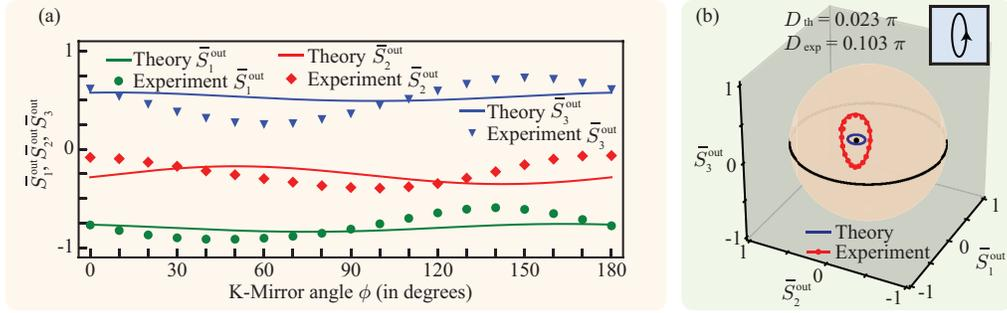
Fig. 7. Experimental plots of normalized Stokes parameters of the transmitted field for an elliptically polarized incident field. (a) Plots of  $\bar{S}_1^{\text{out}}$ ,  $\bar{S}_2^{\text{out}}$ , and  $\bar{S}_3^{\text{out}}$  as a function of  $\phi$ . (b) Poincaré sphere representation of the transmitted field as a function of  $\phi$ .
