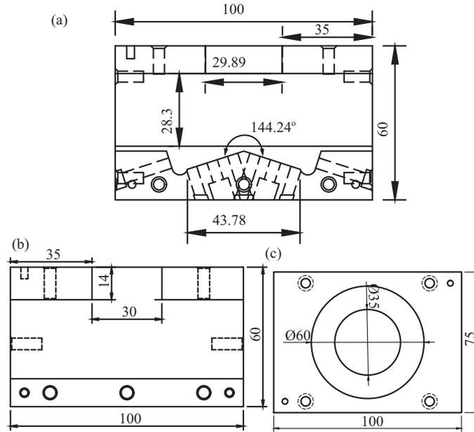
Fig. 4. Design and layout of the K-mirror. (a) CAD drawing of the side-view of the housing. The base of the housing is inclined at an angle  $\beta = 17.88^\circ$  on both sides. (b) CAD drawing of another side-view of the housing. (c) CAD drawing of the top-view of the housing.
