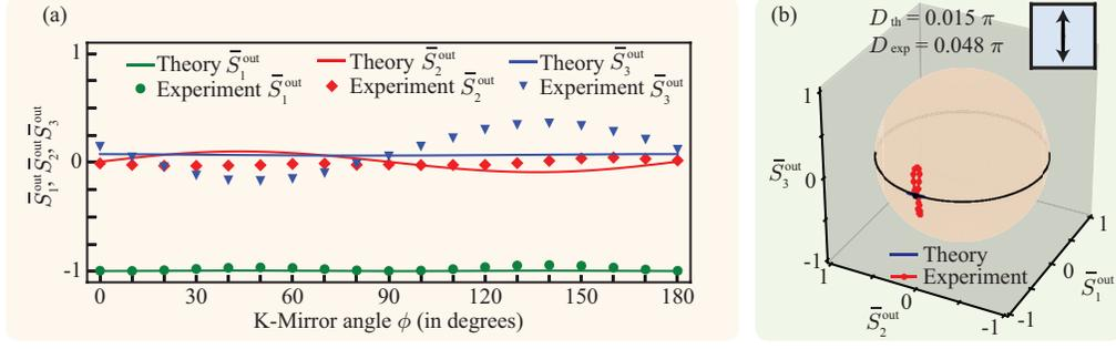
Fig. 6. Experimentally measured normalized Stokes parameters of the transmitted field for a vertically polarized incident field. (a) Plots of  $\bar{S}_1^{\text{out}}$ ,  $\bar{S}_2^{\text{out}}$ , and  $\bar{S}_3^{\text{out}}$  as a function of  $\phi$ . (b) Poincaré sphere representation of the transmitted field as a function of  $\phi$ .
