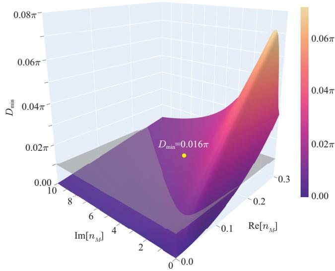
Fig. 3. The minimum mean polarization change  $D_{\min}$ , obtained numerically by optimized over  $\beta$  as a function of  $n_M$ . For a range of  $n_M$  values,  $D_{\min}$  is less than  $0.01\pi$  while for the other  $n_M$  values  $D_{\min}$  is larger than  $0.01\pi$ . The yellow dot represents  $D_{\min}$  corresponding to  $n_M = 0.1568 + 3.8060i$ , the refractive index of the commonly available silver-coating.
